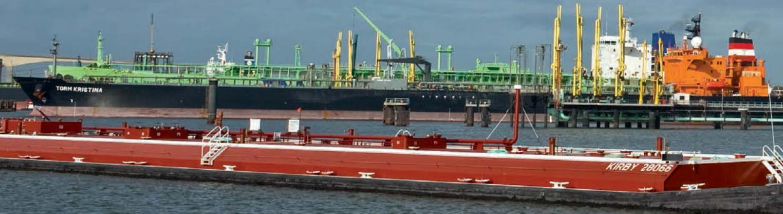
A Kirby Inland Marine tow, the M/V Jeff Montgomery, an 1800 horsepower towboat, with two loaded 30,000 barrel tank barges, transits the Houston Ship Channel.
