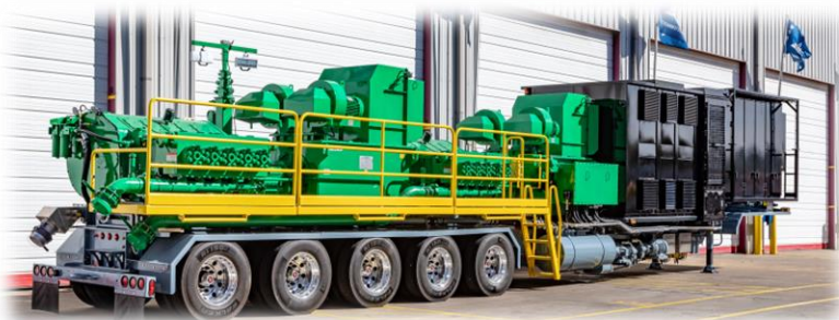
Stewart & Stevenson built electric frac unit
