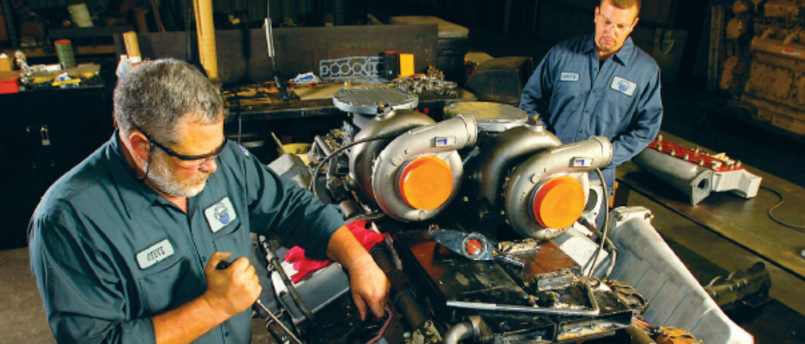
Steve Pellegrin and Corey Bourg rebuild a 1350 horsepower Cummins KT 38 M2 engine from a Gulf of Mexico oil service crewboat.
